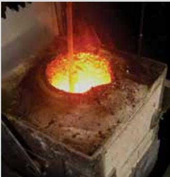
A small pin sample is taken via capillary action through a narrow glass cylinder, called a vacuum pin tube.
