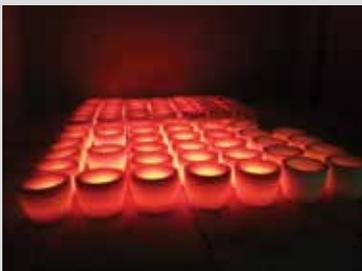
Fire assay is one of the most reliable techniques Scientific Metals uses to assay precious materials.
