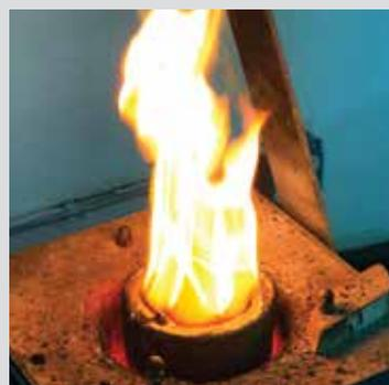
The materials are melted in an induction furnace, which can reach temperatures of more than 3,000 degrees. These high temperatures are necessary to melt platinum and palladium, which have higher melting points than gold.
