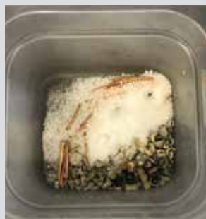
Copper is added to ensure a homogenous melt.
