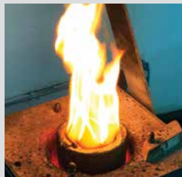
The materials are melted in an induction furnace, which can reach temperatures of more than 3,000 degrees. These high temperatures are necessary to melt platinum and palladium, which have higher melting points than gold.
