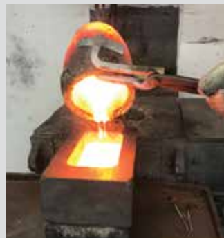
The heated metal is poured from the heated crucible into a bar or ingot mold for cooling, then cleaned and prepped for an after-melt weighing.
